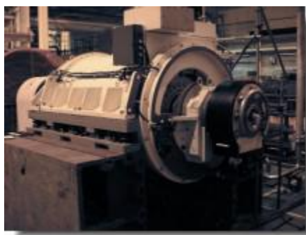
Fig. 7: Motor HTSAC (5 MW – 230 rpm).
