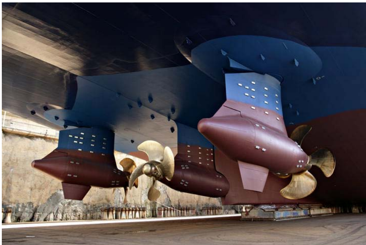
Figure 3.2. Propulsores Azipod's de 14.000 KW cada – Royal Caribbean Cruises
