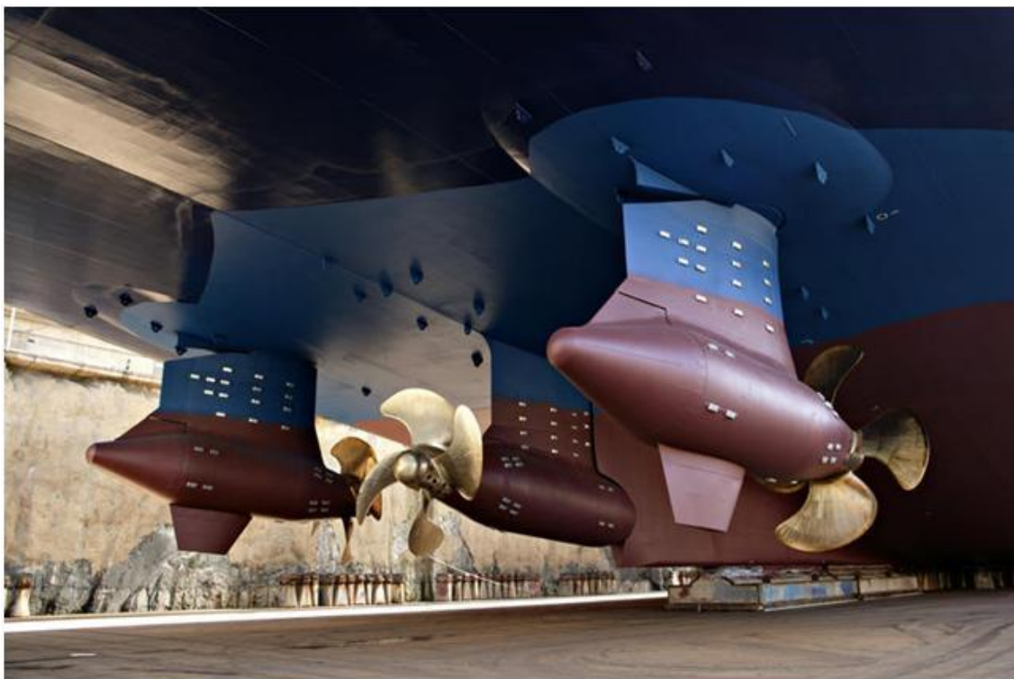
Figura 1. Propulsores AZIPOD'S de 14.000 KW cada – Royal Caribbean Cruises
