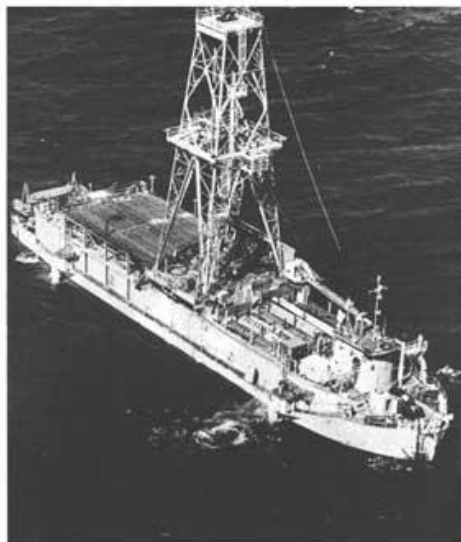
PLATE VI CUSS I during the Guadalupe Island experiments, April 1961. It successfully held position and, for the first time, drilled into the deep-sea floor.
