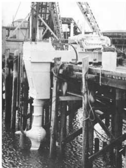
PLATE V Harbormaster 250-hp diesel-powered outboard motor, similar to those which will be used to power CUSS I during the experimental drilling. The engine is fixed but shaft and propeller can turn to exert thrust in any direction.
