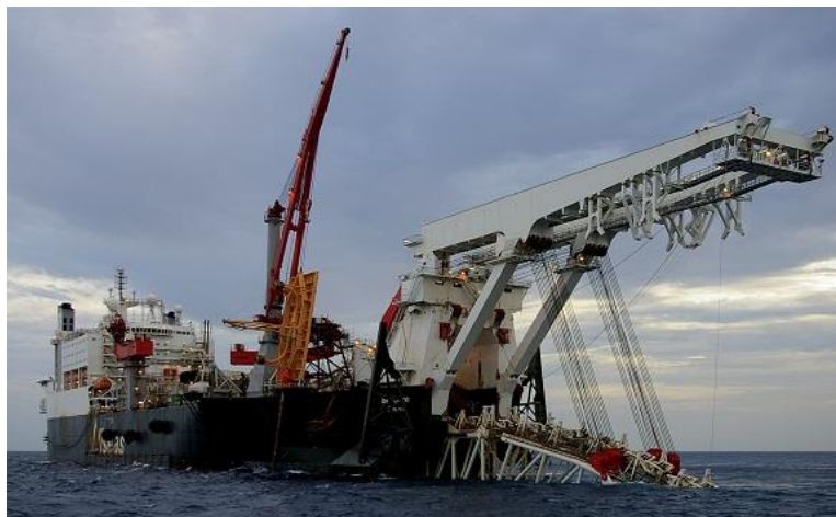
Figura 23 – Pipe Laying Vessel
