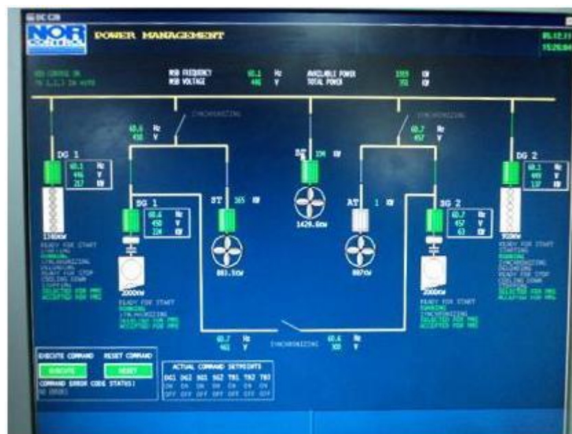
Figura 16: PMS ( Power Management System ).
