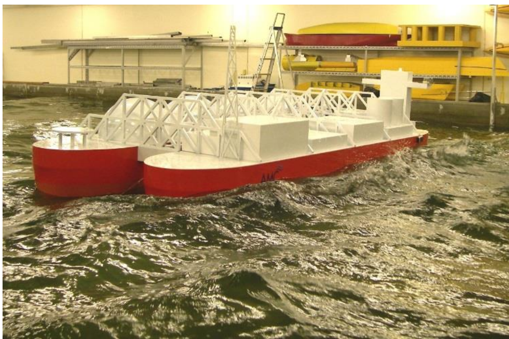
Figura 7 – Tanque de provas com geradores de ondas do Australian Maritime Hydrodynamics Research Centre (AMHRC)
