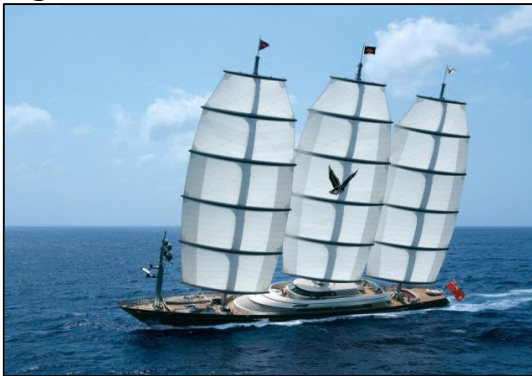
Figura 13: O iate Maltese Falcon usando o Dyna Rig
