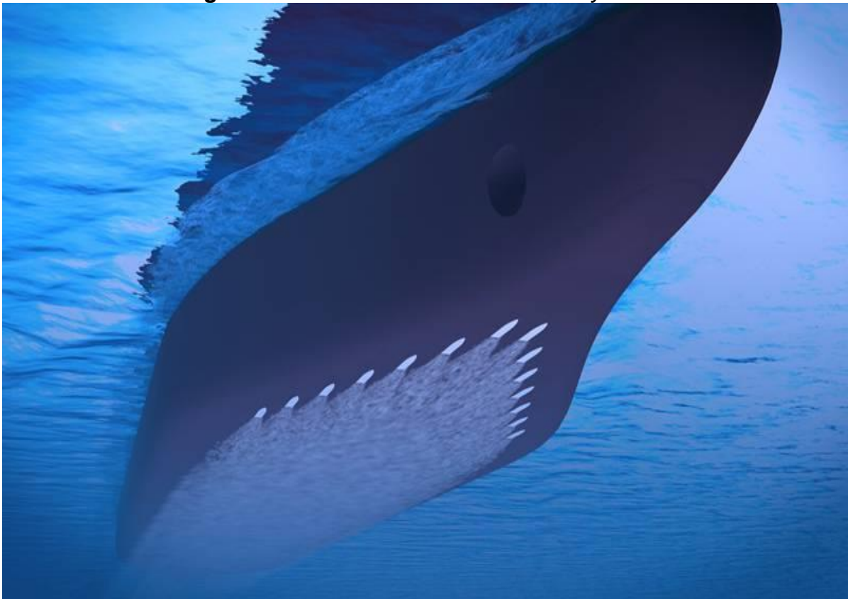
Figura 6 - Silverstream Air Lubrication System
