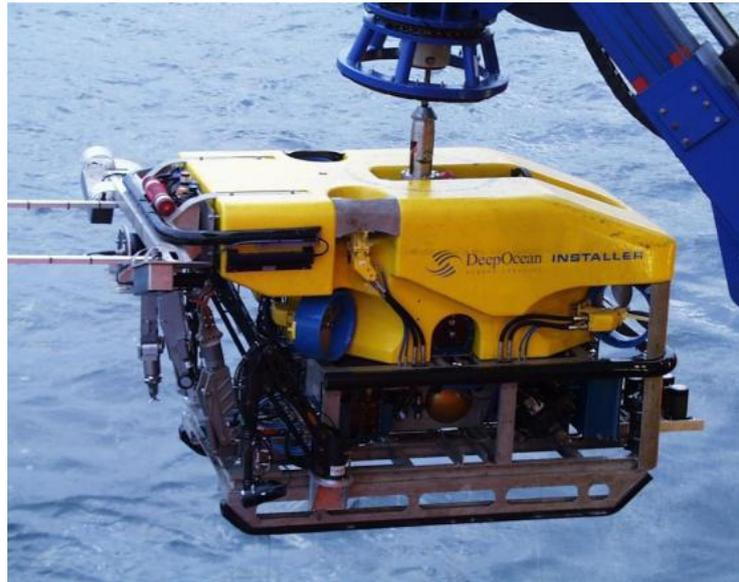
Figura 22 – Installer work class ROV
