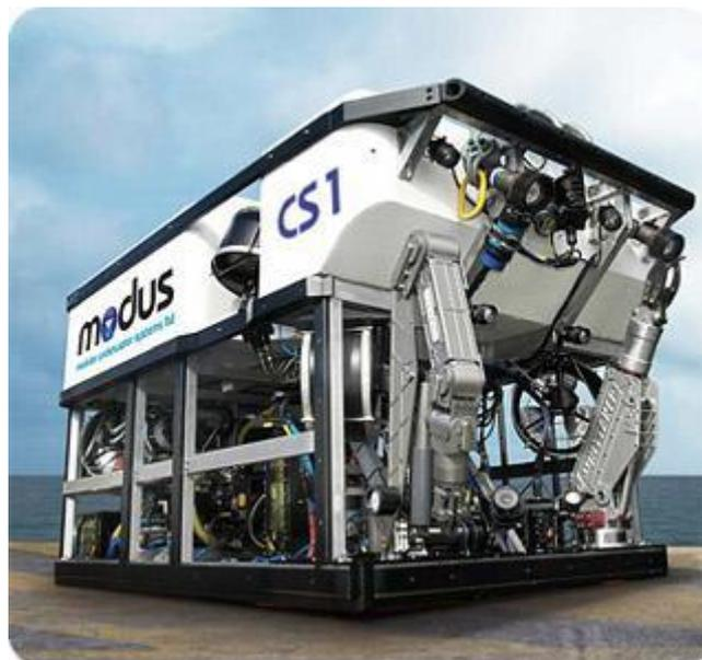
Figura 23 – CS150 construction support ROV
