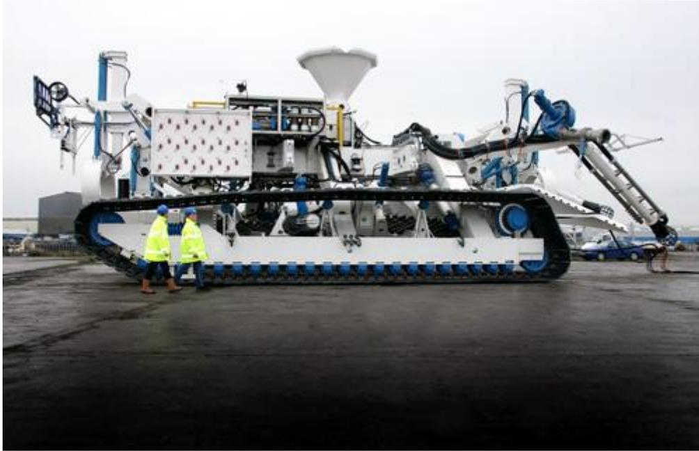
Figura 24 – 2.4MW rock trencher
