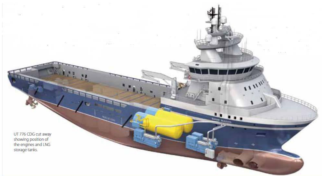
Figura 4. OSV (Offshore Service Vessel) acionado por LNG. Rolls Royce, In Debth, 2011 / Eastlack, 2011.
