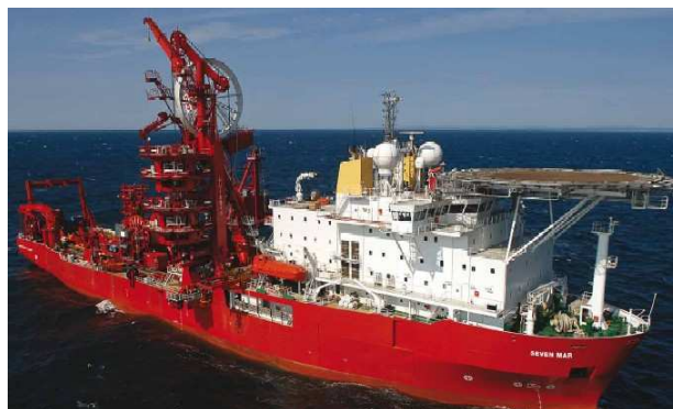
Figura 9: Seven Mar Pipe Laying Support Vessel
