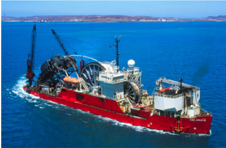
Figura 13 - Pipe Laying Supply Vessel
