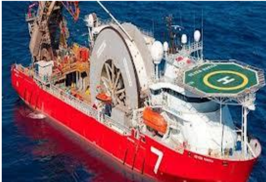
Figura 6: Pipe Laying Supply Vessel
