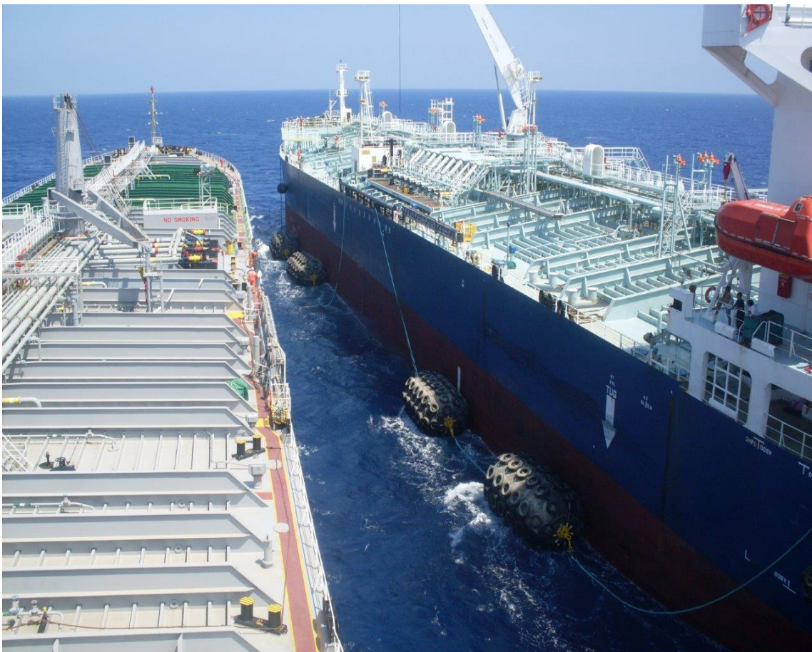
Figura 4 – Operação ship to ship underway
