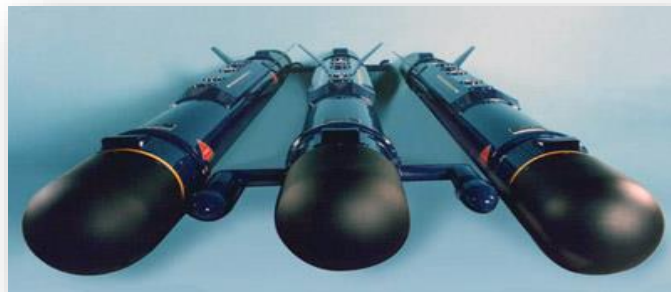
Figura 5.10 - AN/ALQ-167 jamming pods desenvolvido pela Rodale for NATO's Multiservice Electronic Warfare Support Group (MEWSG)
