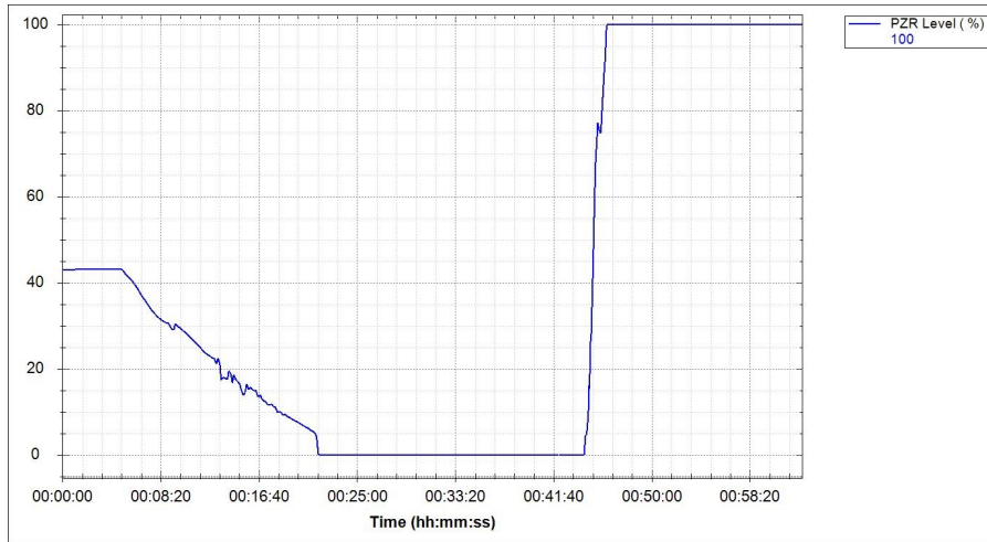
Figure 6.32: PZR level in SGTF transient.
