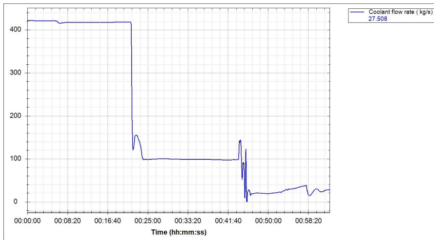
Figure 6.52: RCS coolant flow rate in SGTF transient.
