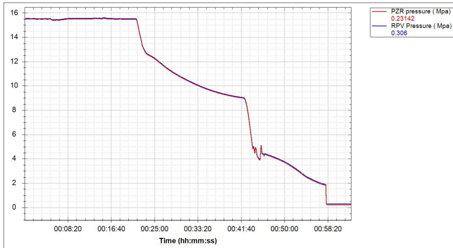
Figure 6.33: PZR and RPV pressures in SGTF transient.
