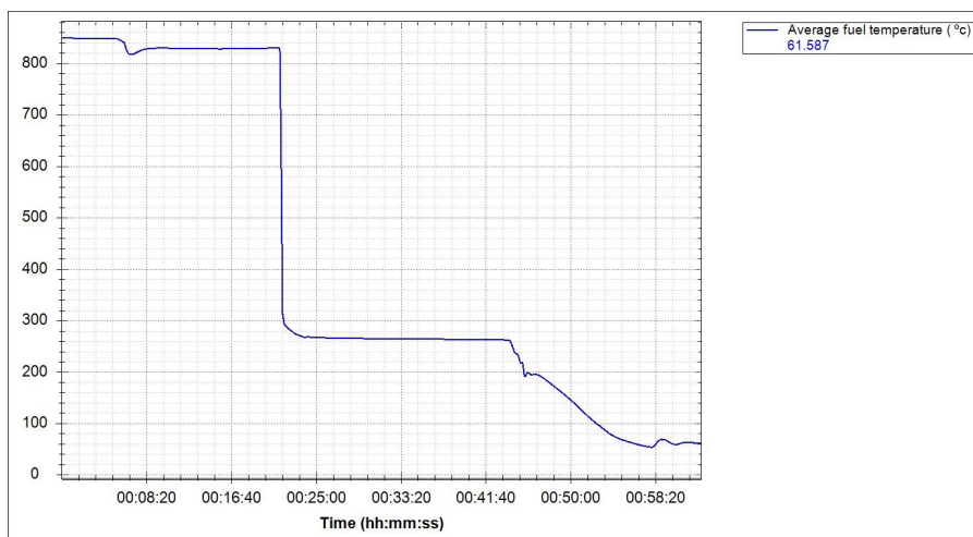
Figure 6.53: Fuel temperature in SGTF transient.
