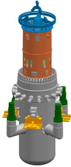
Figure 4.8: ACP-100 reactor with other main equipment connected [7].
