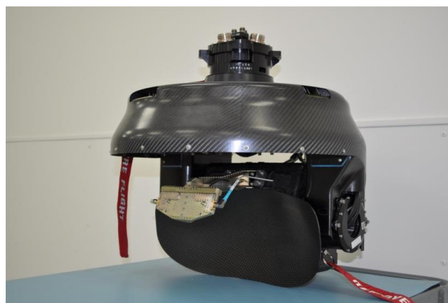
Figura 3.12 – Radar Multi-modo Lynx (GENERAL ATOMICS AERONAUTICAL SYSTEMS, 2017).
