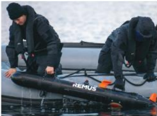
Dutch Navy REMUS Team recovers the Autonomous Underwater Vehicle during Trident Juncture 18. NATO Photo By WO FRAN C Valverde
