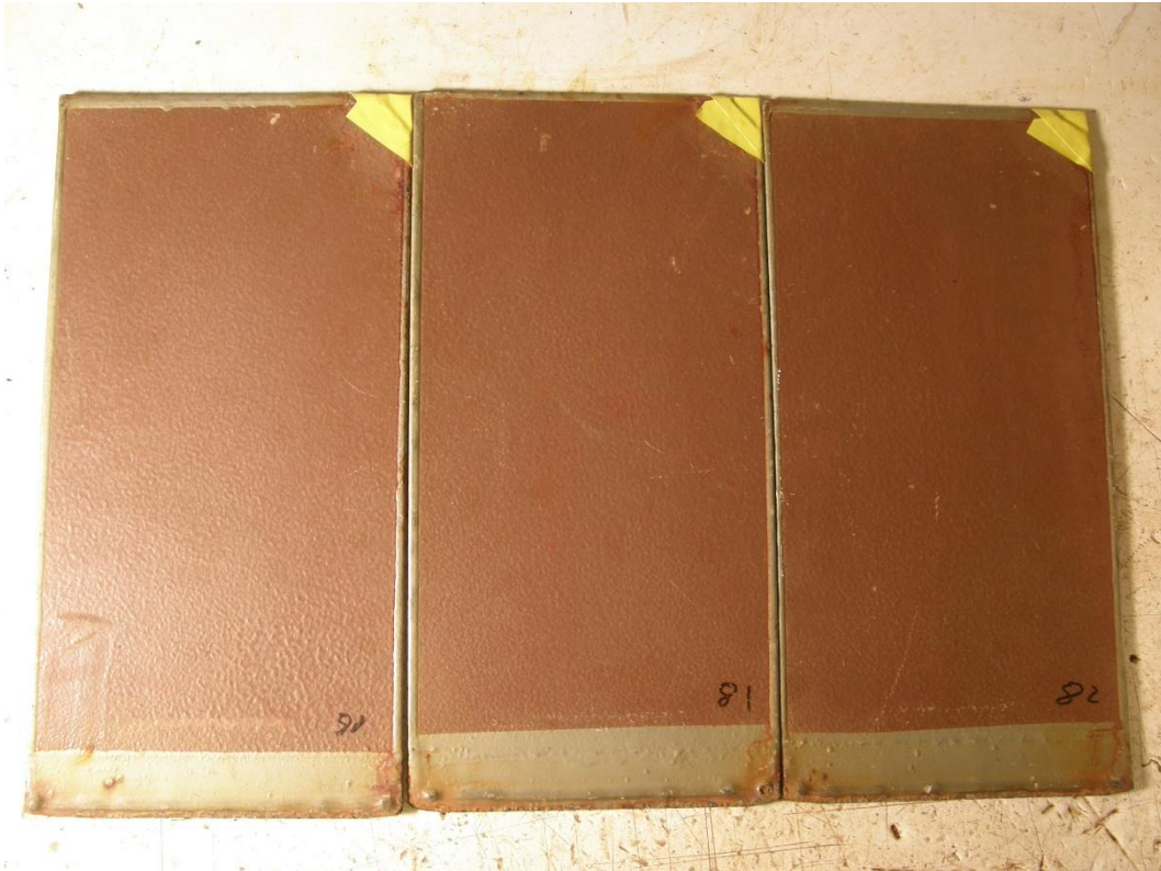
Figure 3.18 – Coating D panels at week 101 (opposite side).
