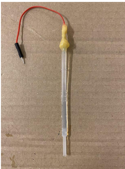
Figure 3.27 – Reference electrode prepared for the electrochemical experiments.
