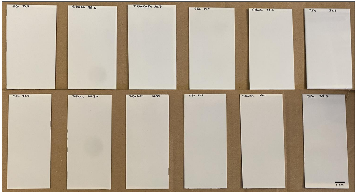
Figure 3.6 – Model coatings on aluminium alloy (on top) and mild steel (below) substrates.
