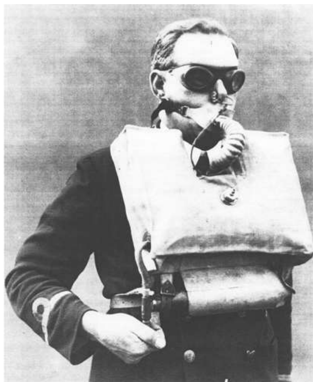
Davis Submerged Escape Apparatus (D.S.E.A.)
