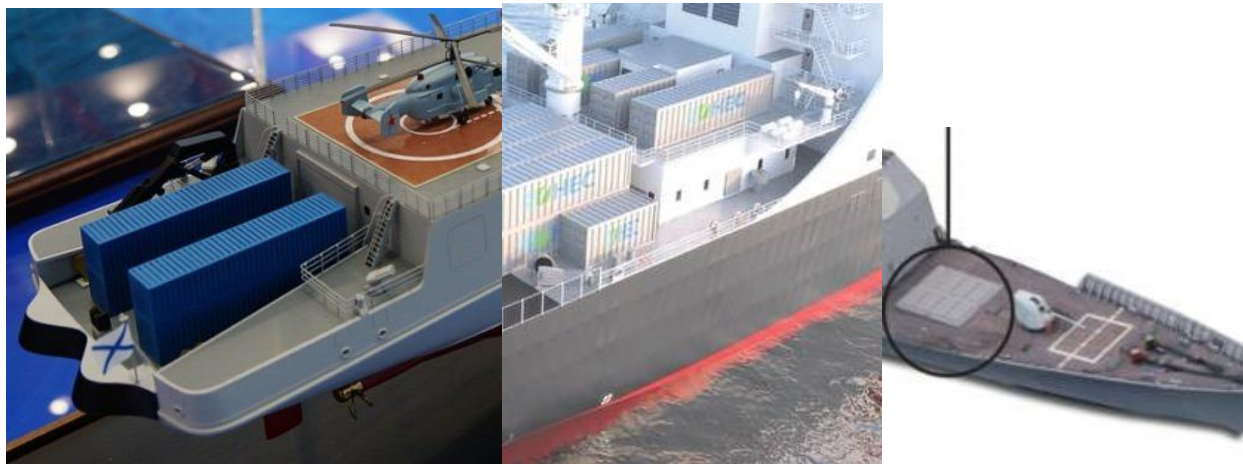
Figure 24 – Stern 14 , Midship 15 and Forward 16 Modules Slots Location
