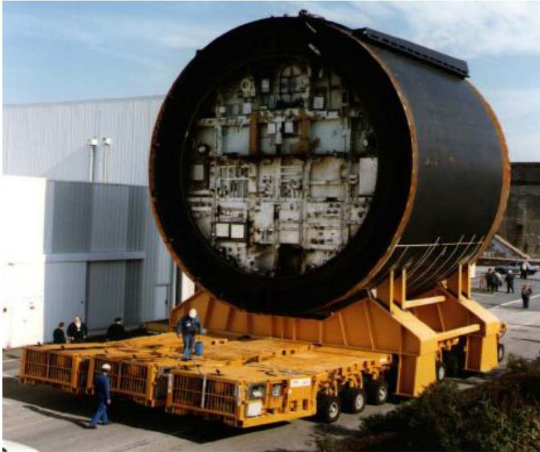
Figure 8 - French NS class “Le Redoutable” reactor compartment transportation
