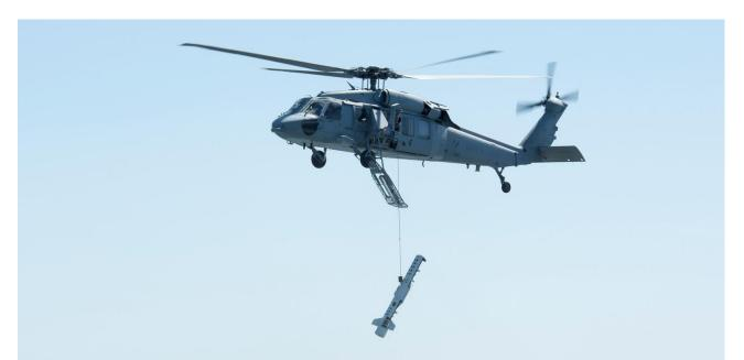
18. The neutralizer vehicle is released from the LHS under the control of the sensor operator on the aircraft. The operator guides the lightweight (15.5 kg) and highly maneuverable vehicle to the target location using on-board sonar. After the target is viewed and positively identified with an on-board video camera, the operator fires an armor-piercing warhead from the vehicle to neutralize the mine. The neutralizer's state-of-the art electronics and sensors also provide a robust,
