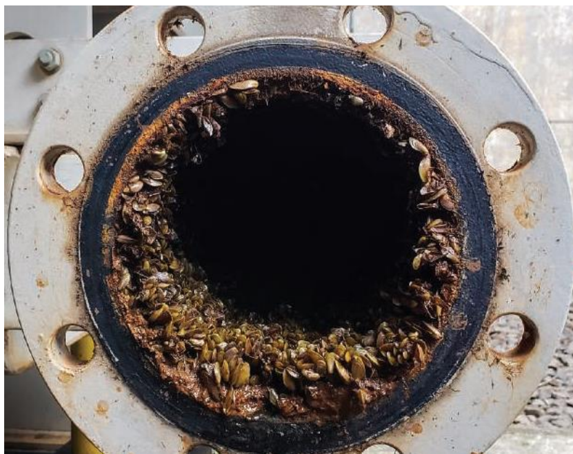
Figura 5 – Mexilhão dourado ( Limnoperna fortunei ) obstruindo duto de usina hidroelétrica. Fonte: Moutinho, S. 2021. A Golden Menace - An invasive mussel is devastating ecosystems as it spreads through South American rivers, threatening the Amazon basin. Science.
