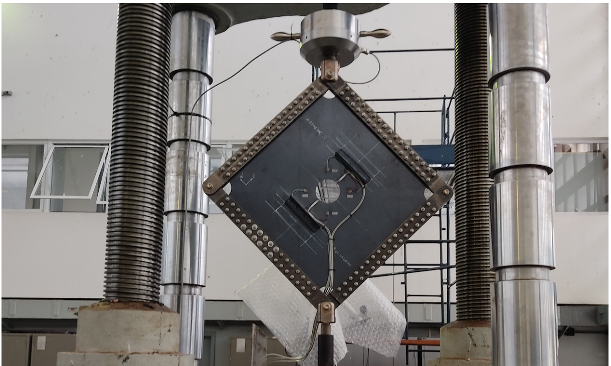
FIGURE 6.7 – Figure obtained from a photograph captured in the structural laboratory of ITA, showcasing the setup apparatus, including the assembly of the panel and picture frame on the testing apparatus during the tests.
