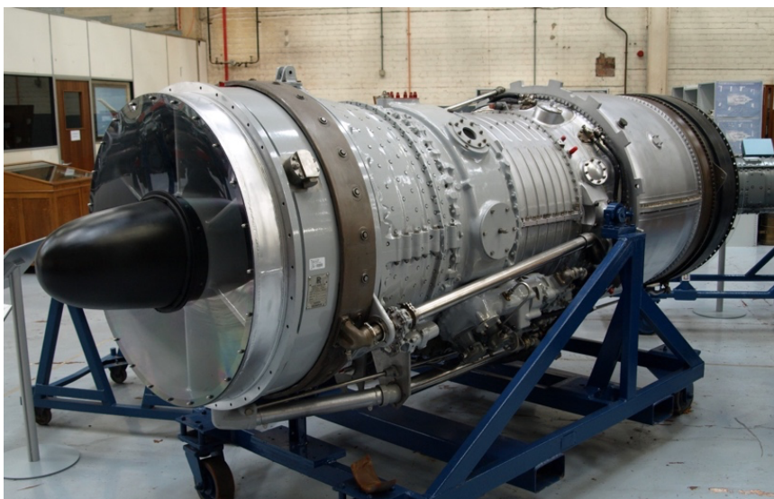
Figura 24 - Turbina Olympus TM3B.
